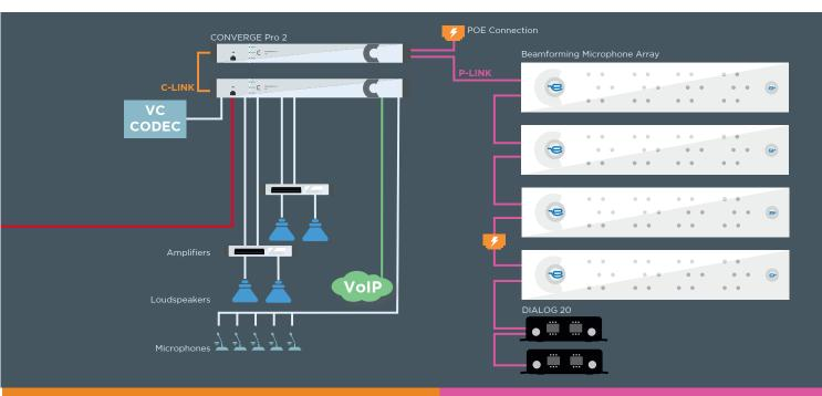
**C-LINK** gives you a scalable system. Units can be stacked together in any combination
